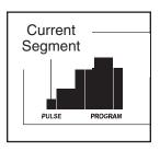
several segments will be shown in the columns to the right. When only three seconds remain in the first segment of the program, both the Current Segment column and the column to the right will flash and a series of tones will sound. When the first segment ends, all target heart rate settings will move one column to the left. The target heart rate setting for the second segment will then be shown in the flashing Current Segment column.
